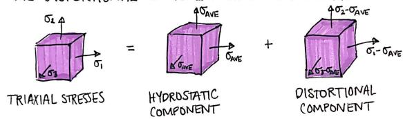
THE DE THEORY SUGGESTS THAT IT IS THE DISTORTIONAL COMPONENT THAT LEADS TO FAILURE. THE FAILURE CRITERION IS
